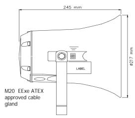
Bracket and all outside nuts and screws in stainless steel.
