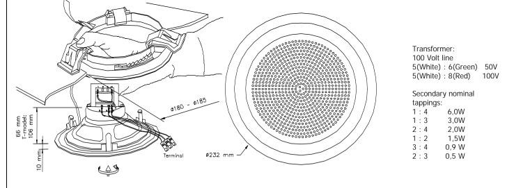
Rec. ceiling hole: ø180 - ø185 mm
