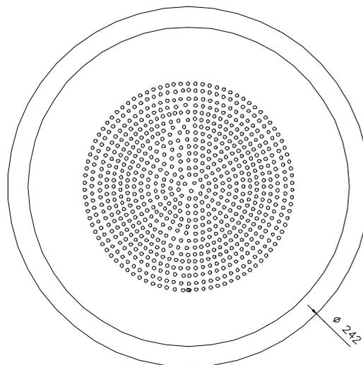
Rec. ceiling hole:  $\varnothing$  167 mm
