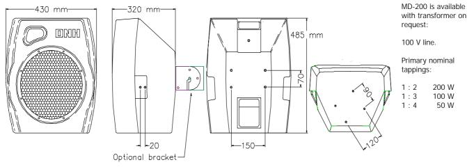
MD-200 is supplied with M8 stainless steel threaded inserts for mounting purposes. Deviation from the given mounting-hole dimensions might be  $\pm$  2 mm.
