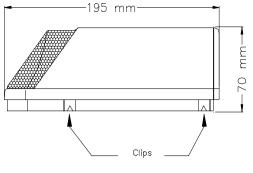
Remove the lid by pressing the two clips on each side of the loudspeaker 50 V /100 V combined transformer:
